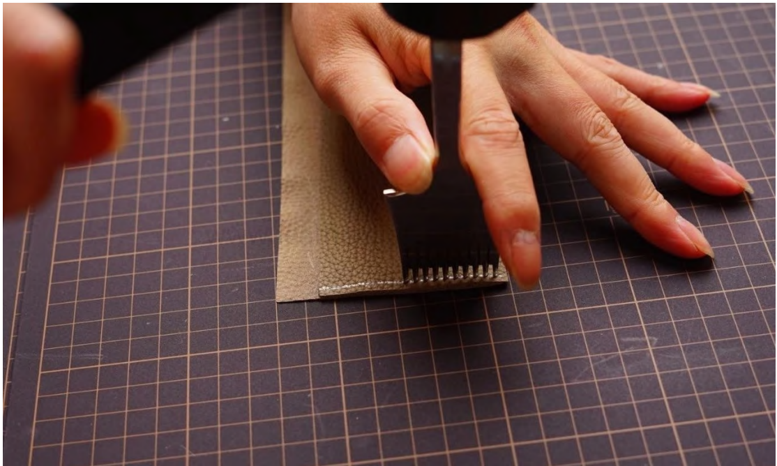
Step 89: Punch chisel holes.
