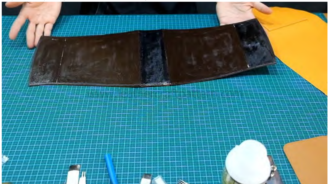
Step 15: Full paint glue on surface and lining.
