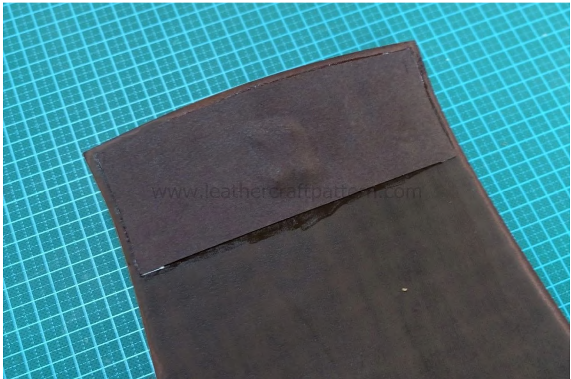
Step 15: Full paint glue on surface and lining.
